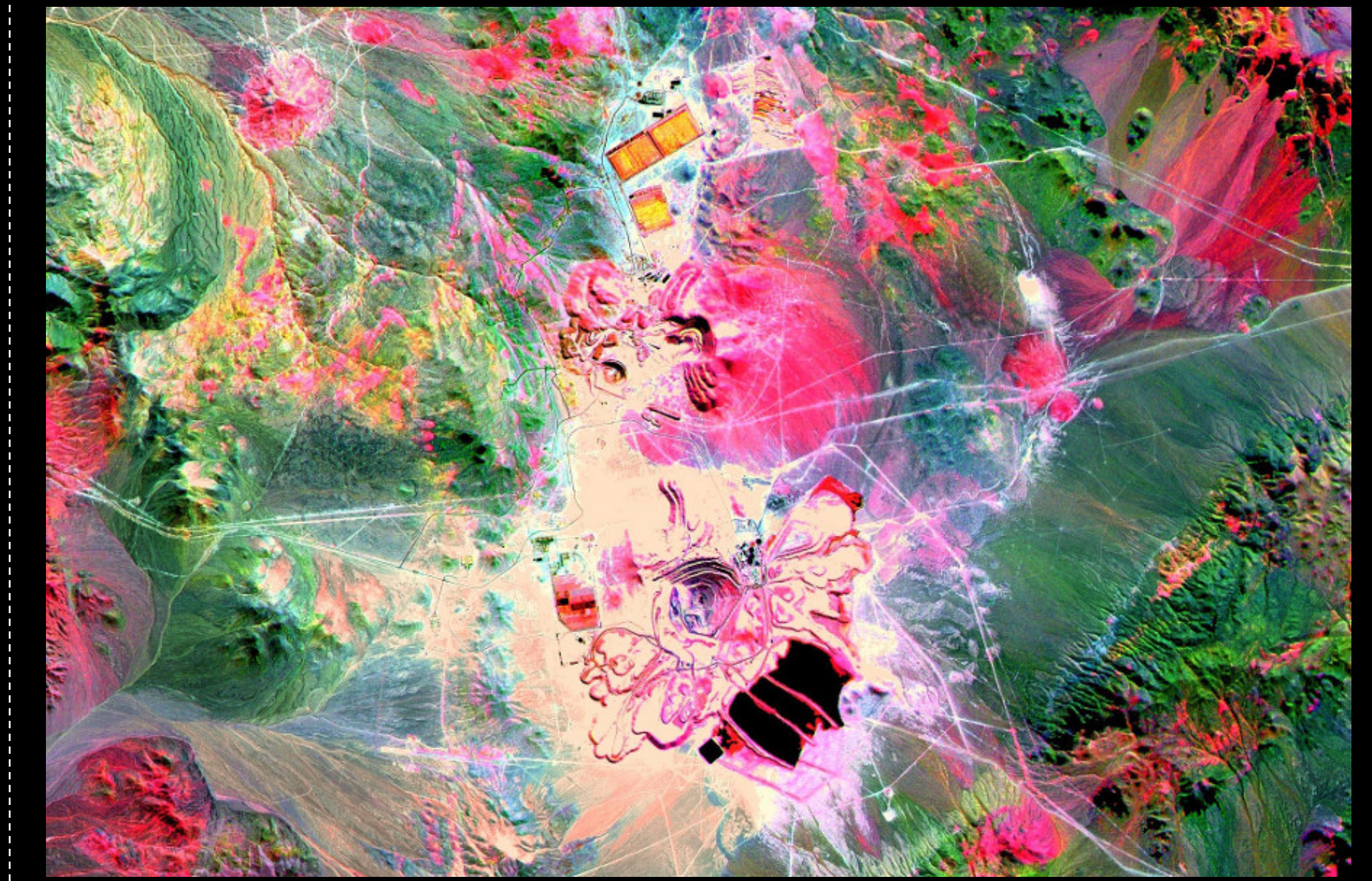
Hyperspectral imagery of the Escondida Mine in Chile. Courtesy NASA/JPL-Caltech.
